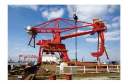
The capacity is 1000-4500t/h. Applicable to the vessel type of 35000~40000DWT. The higher vessel capacity, the more obvious discharging efficient strength.
